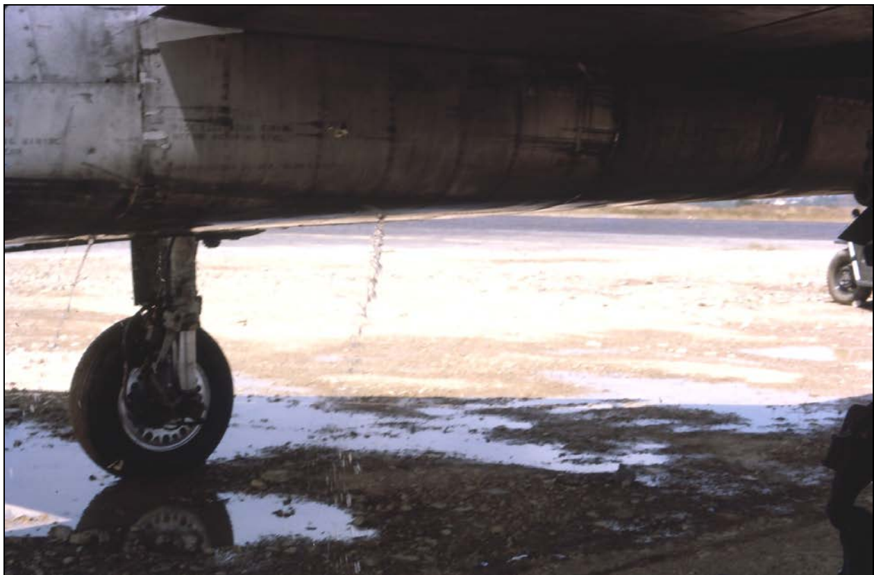
With fuel streaming from bullet holes, the pilot had just a few minutes to get the plane back on the ground. Our Caribous were frequently hit by ground fire but fortunately the 'Bou' could take a lot of hits and still keep going.
