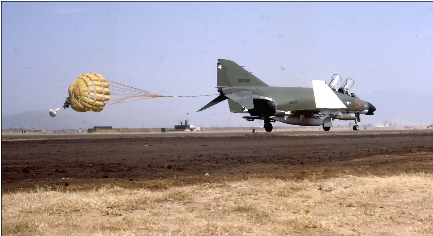
Heavy US Navy Phantom uses drag chute to help slow down on landing at Phan Rang.
