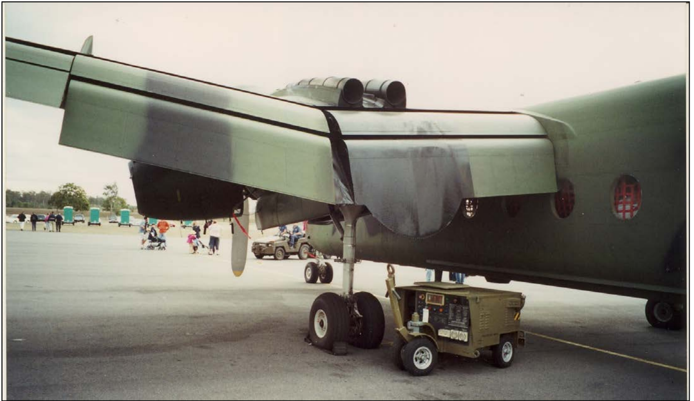
This pic shows the Caribou's huge double-slotted flaps and double-slotted drooping ailerons. (Note exhaust augmentor tubes on top of the wing)
