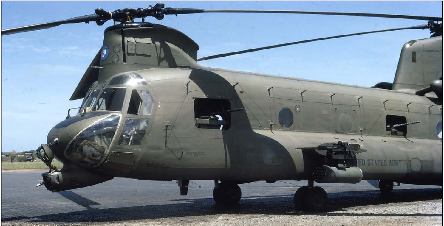
“Guns-a-Go-Go” heavily armoured Chinook gunship. Chin-mounted grenade launcher, side-mounted cannons and rocket pods, side and rear firing 50 cal. machine guns.
