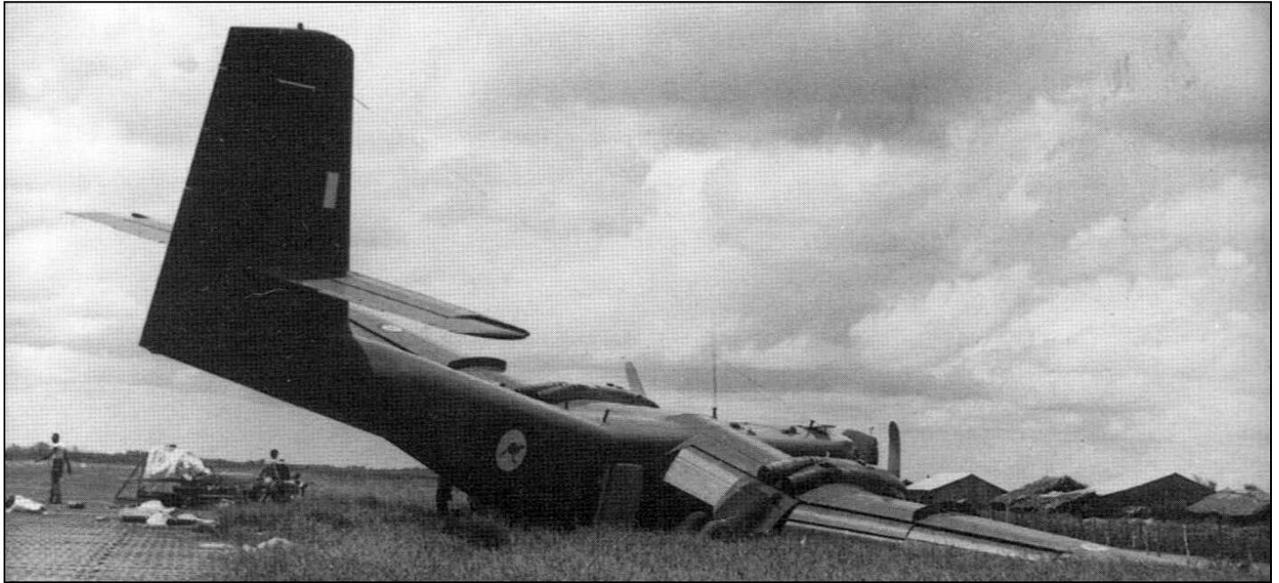
A4-173 in its resting place after landing short and running off the strip at Hai Yen on 7 May 1965. The accident required a major repair effort involving replacement of the wing, undercarriage, propeller and other components. The aircraft flew out under its own power four days later, and after being rebuilt was back in service by September.
