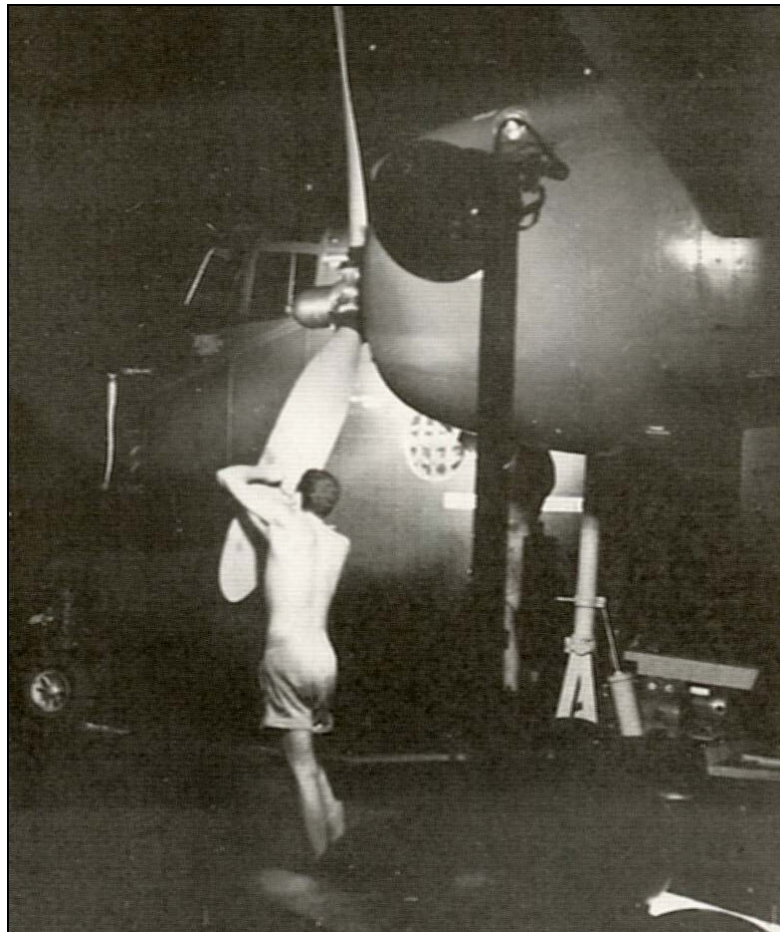
John McDougall repairing stone damage to Caribou propeller. RTFV/35 SQN ground crews worked 24-7 to keep aircraft on the line.
