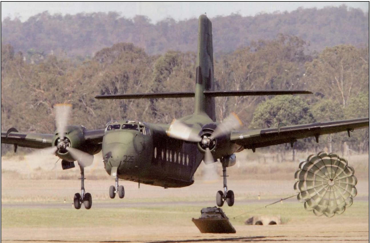
The LOLEX low level extraction is now called LAPES – low altitude parachute extraction system. It is used where a heavy load has to be delivered accurately to a relatively open and level drop zone.
