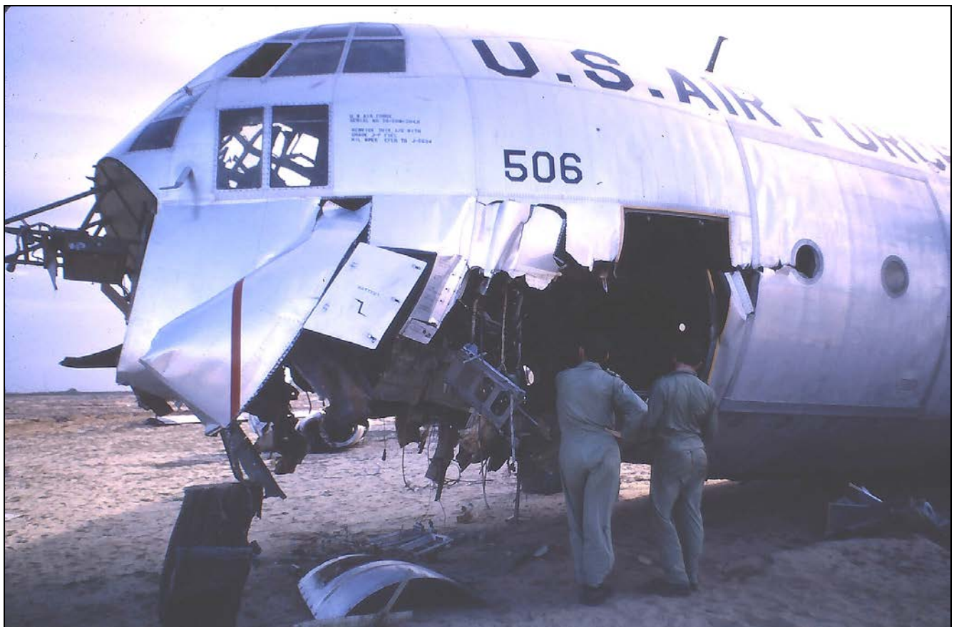
Result of US Army's ham-fisted attempt to drag bogged Herc out of the sand.
