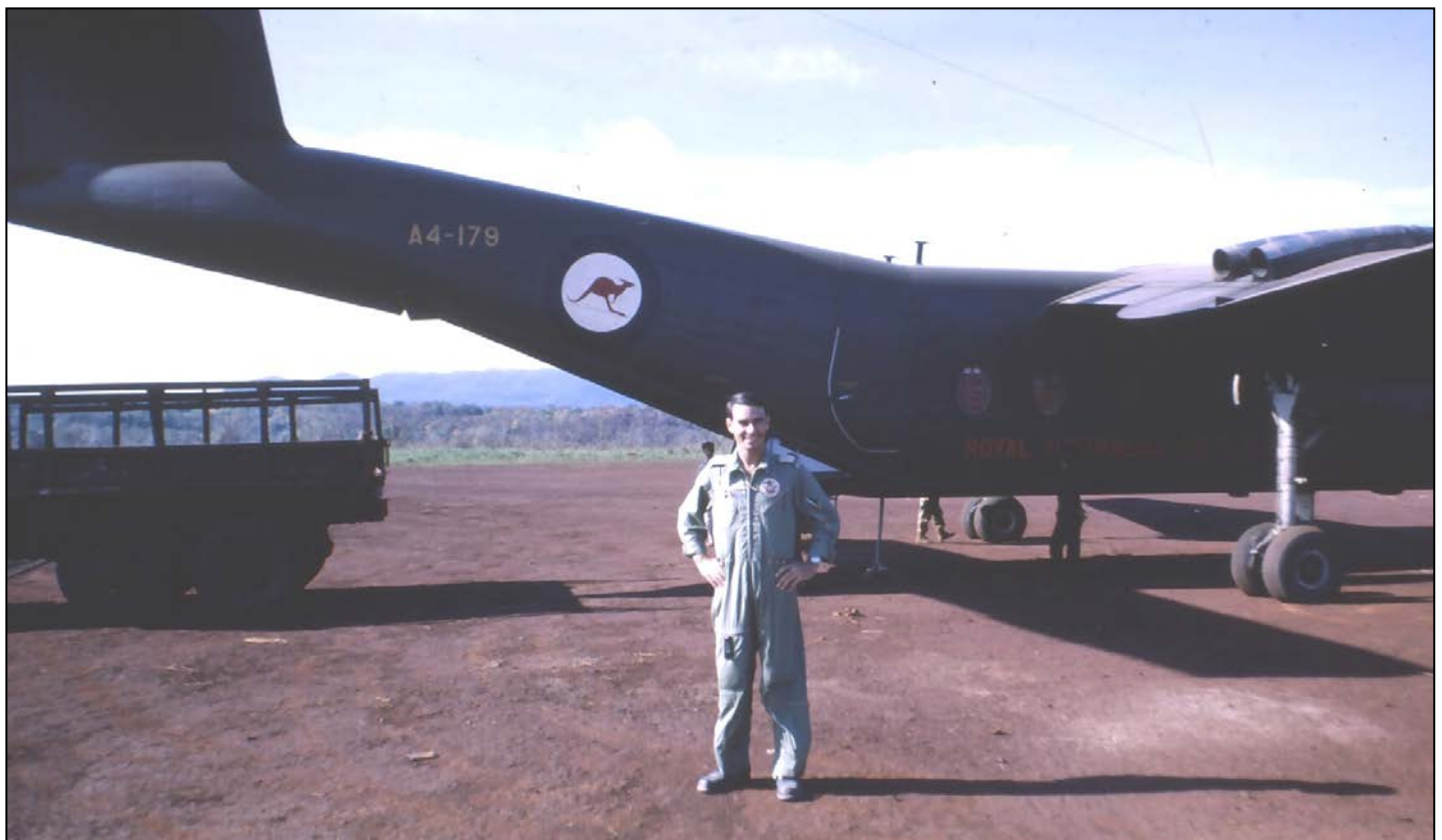
This pic shows the Caribou's huge double-slotted flaps and double-slotted drooping ailerons. (Note exhaust augmentor tubes on top of the wing)
