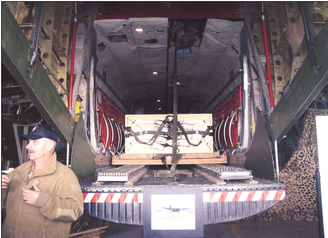
The rather complex 'LAPES' set-up as displayed by AMTDU at Richmond. Package sits on a crushable cardboard honeycomb base designed to absorb the impact of the six foot drop.
